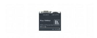
The PT-110 is a twisted pair transmitter for computer graphics video signals. It converts a computer graphics signal into a twisted pair signal which is converted back to a computer graphics video signal when used in conjunction with the Kramer TP-120 twisted pair receiver (or other compatible Kramer receiver).
